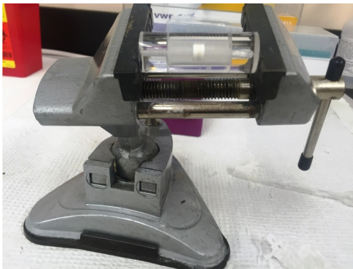
Figure 5-6 Photograph showing the compression chamber based on the schematic in Figure 5-5 . Tissues were loaded between two porous plates in order for the water that is exuded during compression to be absorbed.
